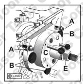
Check installation position of timing ring on crankshaft again (refer to page 13).
