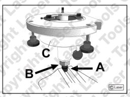
Before fitting the new seal housing, check that the hole in the timing ring is aligned with the TDC mark on the seal housing. A plastic clip (ARROW) holds the ring in the correct position, this must be removed.
