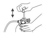
Pressurise the tank by pumping handle (D) up and down; take care not to let the pressure exceed 20psi.
