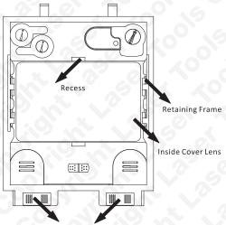
Replace the inside cover lens if it is damaged (cracked, scratched, pitted or dirty). Remove the old front cover lens by pressing two Lock Switches at the bottom of the Retaining Frame and pull the frame and ADF out. Take the old front cover lens out, and remove any protective film before installing the new one.
