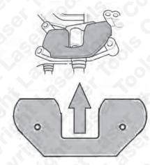
**Component B** – Balance Shaft Locking Tool Used to lock the balance shafts. Install as shown.
