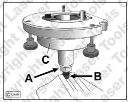
Before fitting the new seal housing, check that the hole in the timing ring is aligned with the TDC mark on the seal housing. A plastic clip (**A**) holds the ring in the correct position, this must be removed. Locating hole **B** on timing ring **C** must align with TDC mark **A** on seal housing.
