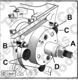
Check installation position of timing ring on crankshaft again (refer to page 13). If dimension -a- is too small again, tighten large hex nut **A** to to **45 Nm** using torque wrench and check installation position of timing ring on crankshaft again.
