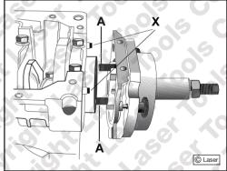
NOTE: Screw Allen-headed bolts **A** into crankshaft flange (approximately 5 full turns).
