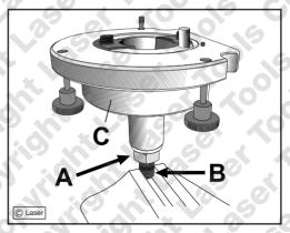
Before fitting the new seal housing, check that the hole in the timing ring is aligned with the TDC mark on the seal housing. A plastic clip (A) holds the ring in the correct position, this must be removed.
