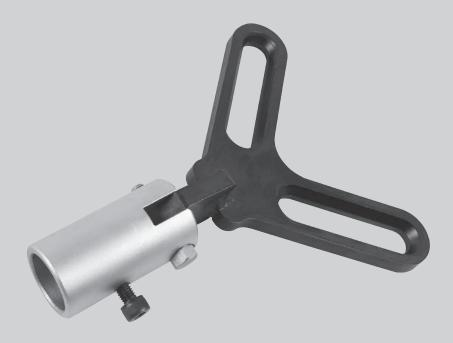
• Designed to fit on top of a standard hydraulic transmission jack and convert the jack into a Hub Support device. This allows load to be applied vertically to the hub to assist in the separation of the bottom ball joint, etc. the jack can then take the load of the drive flange, hub and suspension strut assembly while the lower arm etc. are worked on. Particularly use full when working on vehicles with restricted suspension droop.
