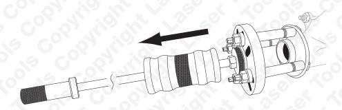
Refer to diagram above and assemble as shown. Driveshaft / CV joint has previously been removed. Assemble hammer weight **(H)** onto slide hammer shaft **(B)** then screw shaft tightly into adaptor **(G)**. Tighten shaft
