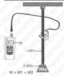
A feature of the Laser 5846 is its ability to be easily recalibrated by the user.
