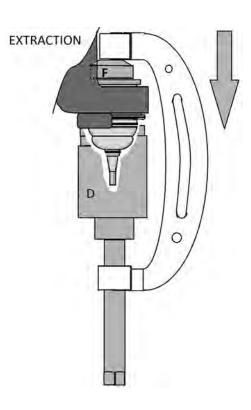
Assemble on the top arm as shown with the force screw pushing up. Using a socket and ratchet only wind the ball joint out.
