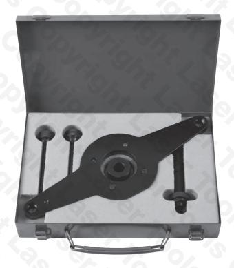
This is an essential item required to maintain the engine timing when removing the front vibration damper.
