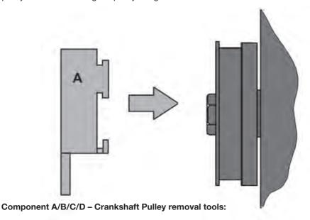
Use components A, B, C & D to draw off the crankshaft pulley after the pulley bolt has been removed.
