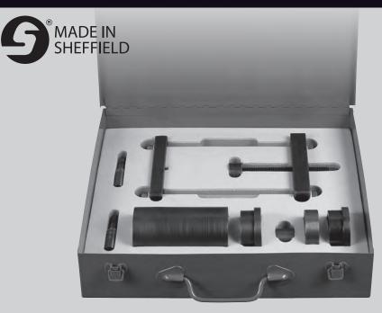
This kit has been design specifically to remove and fit the bottom ball joints fitted to the Land Rover Discovery 3-4 series and Range Rover Sport. The kit allows the bottom ball joint to be replaced and fitted without removing the lower wishbone assembly.
