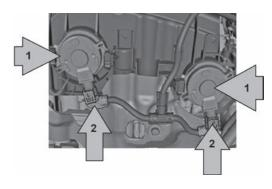
Place the 7329 on to the actuator as shown in Fig. 2 and turn the actuator through approximately 50°. Remove actuator.
