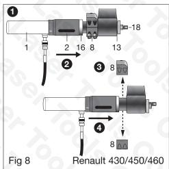
Refer to **Figure 8** and fit bush clamp (8) to insertion tool, then complete tool assembly to spring eye (**operation 1**). Operate hydraulic pump to start inserting bush into spring eye (**operation 2**). Remove bush clamp (**operation 3**), then operate hydraulic pump to fully fit the bush (**operation 4**).
