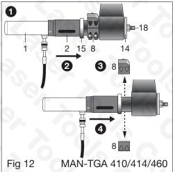
Refer to **Figure 12** and fit bush clamp (8) to insertion tool, then complete tool assembly to spring eye (**operation 1**). Operate hydraulic pump to start inserting bush into spring eye (**operation 2**). Remove bush clamp (**operation 3**), then operate hydraulic pump to fully fit the bush (**operation 4**).
