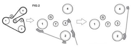
•Always check the pulleys in 2 positions as shown in figure 3 to check for angular misalignment.
