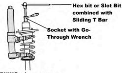
WARNING: always use appropriate spring compressor before removing top fixings
