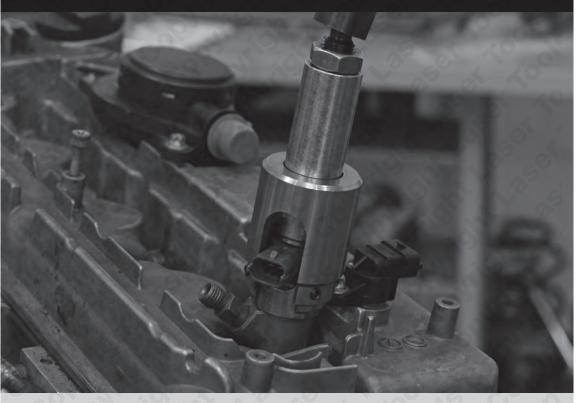
The 7802 adaptor has been designed to allow the extraction of Bosch CR Solenoid style diesel injectors without the need to remove the injector solenoid or internals.
