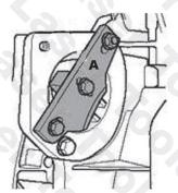
**Components A:** Used to lock the flywheel when loosening and tightening the crankshaft pulley bolt. Remove the starter motor, assemble components A as shown and fit in the starter aperture so that its tooth locks the flywheel.
