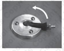
**1.** Slightly loosen screws on back plate to release connector.
