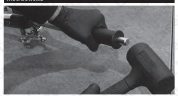
Step 3: Gripping the handle firmly, tap the head of the Driver Pin with a Dead Blow Hammer until it bottoms out.
