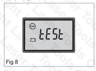
Press enter button (4) to begin the test. The display will initially show the measured voltage (Figure 9):
