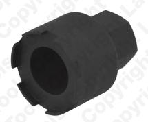
Special socket designed for the removal and installation of the oil pressure control solenoid switch found on the Mercedes M651 diesel engines. The M651 engine is found across the Mercedes-Benz car and van ranges. Can be used with a 24mm spanner or 1/2"D socketry as access allows.
